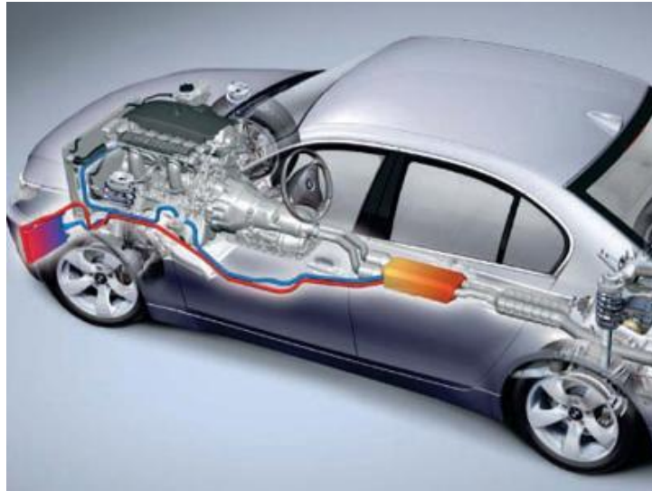
Figure 1.1.1 Thermoelectric generator incorporated in a car design. Figure reproduced from reference 2
